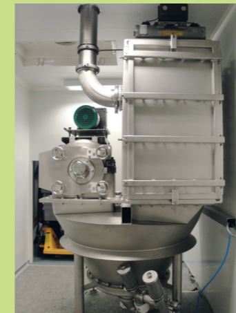
Grinding mill with filter for pharmaceutical, explosion proof, CIP
