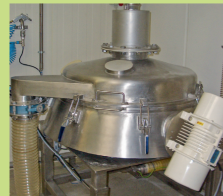
Inline sifter GSC900 in suction conveying in food branch
