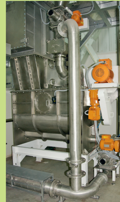
Sugar mill with filter and receptacle explosion proof
